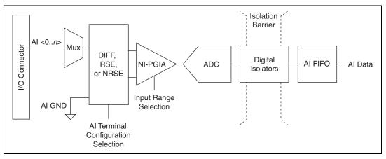
Figure 4-1 shows the analog input circuitry of NI 6232/6233 devices.
